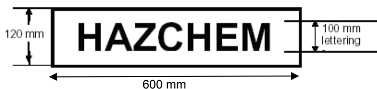
Figure 13.1 Form and dimensions of outer warning placard
